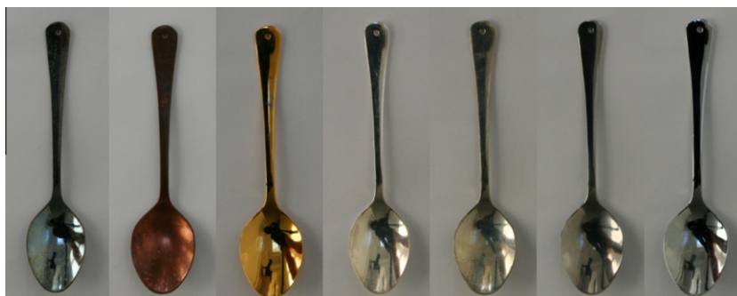
Fig. 1. The spoons used in the study are pictured. They are stainless steel spoons electroplated with the following metals (from left to right): zinc, copper, gold, silver, tin, stainless steel and chrome.
